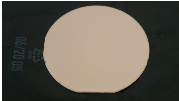
wafer with 100:1 mix ratio after sputtering
