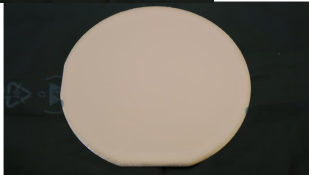
wafer with 50:1 mix ratio after sputtering
