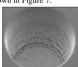
**Figure 7** Fully-sloped and veil free via
